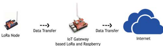
Fig. 3. Architecture Of Environment LoRa Network to Internet
